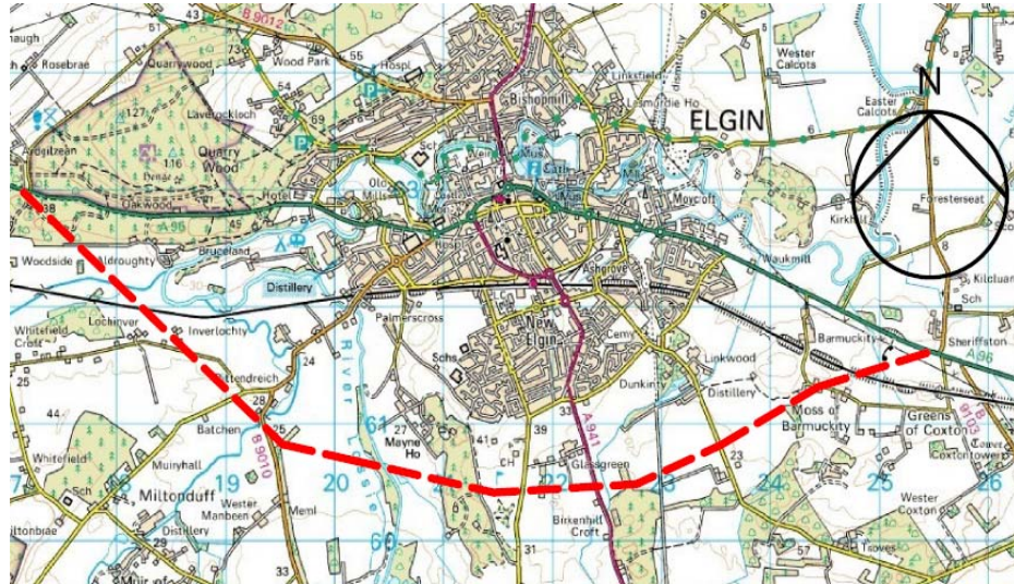
Figure 5.2: Assumed Bypass Route Alignment for Elgin
