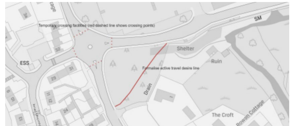
Temporary lights-controlled crossing points on junction to improve pedestrian safety at current advisory crossings Improve earth-beaten desire line path with compacted hardcore or equivalent
